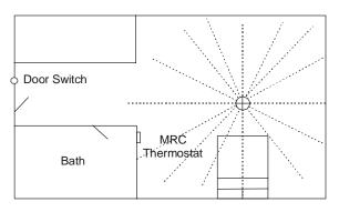
Figure 7: Ceiling Mount PIR Field of Coverage
