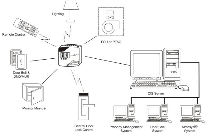
Figure 2: System Components
