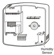
Figure 5: Humidity Sensor Location
